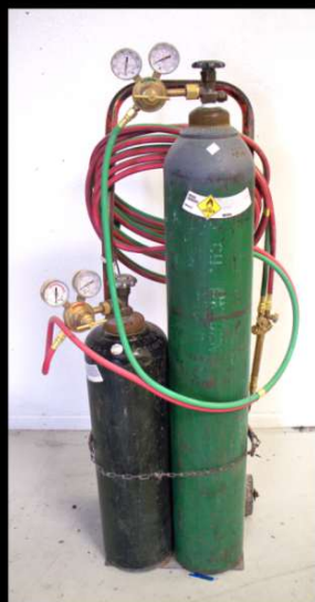
Gas welders and cutting torches
