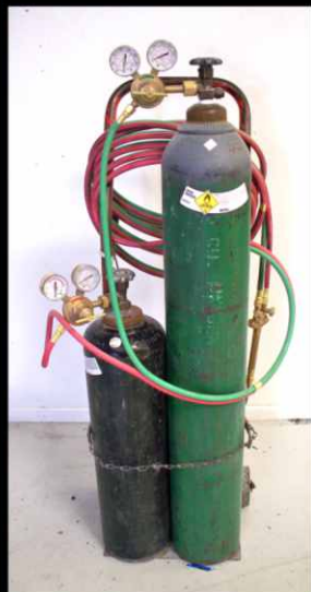
Gas welders and cutting torches
